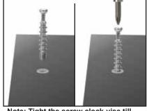
Note: Tight the screw clock-vise till the thread disappear.
