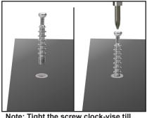
Note: Tight the screw clock-vise till the thread disappear.
