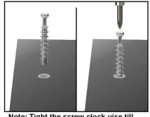
Note: Tight the screw clock-vise till the thread disappear.
