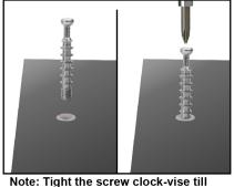
Note: Tight the screw clock-vise til the thread disappear.
